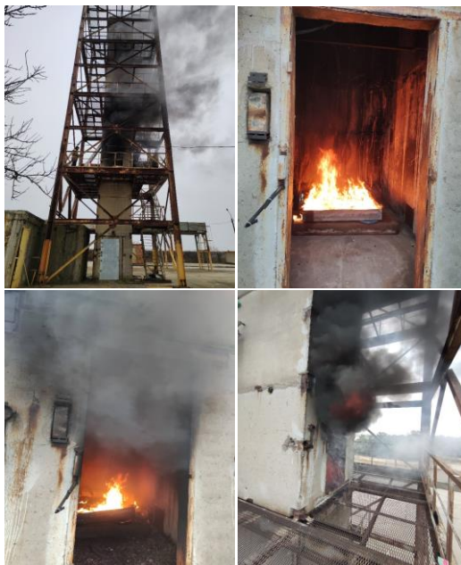
Fig. 1 - Cable tunnel of the NPP during the experiment.
