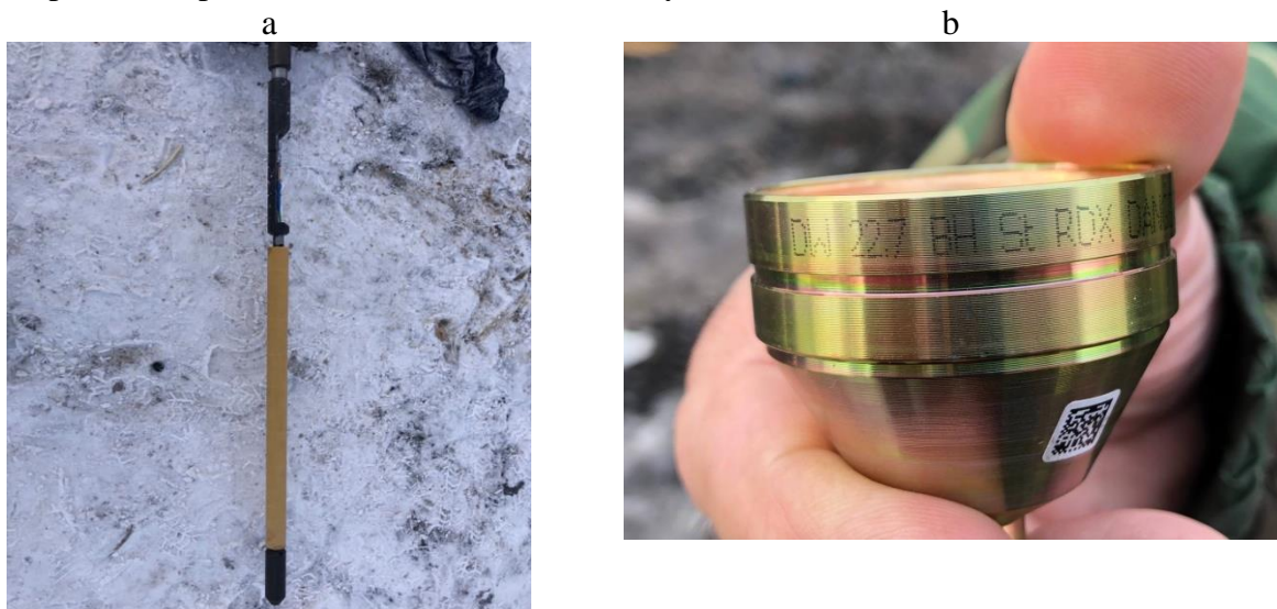
Figure 1 – Cumulative PNKT perforator (a) and charge (b)
